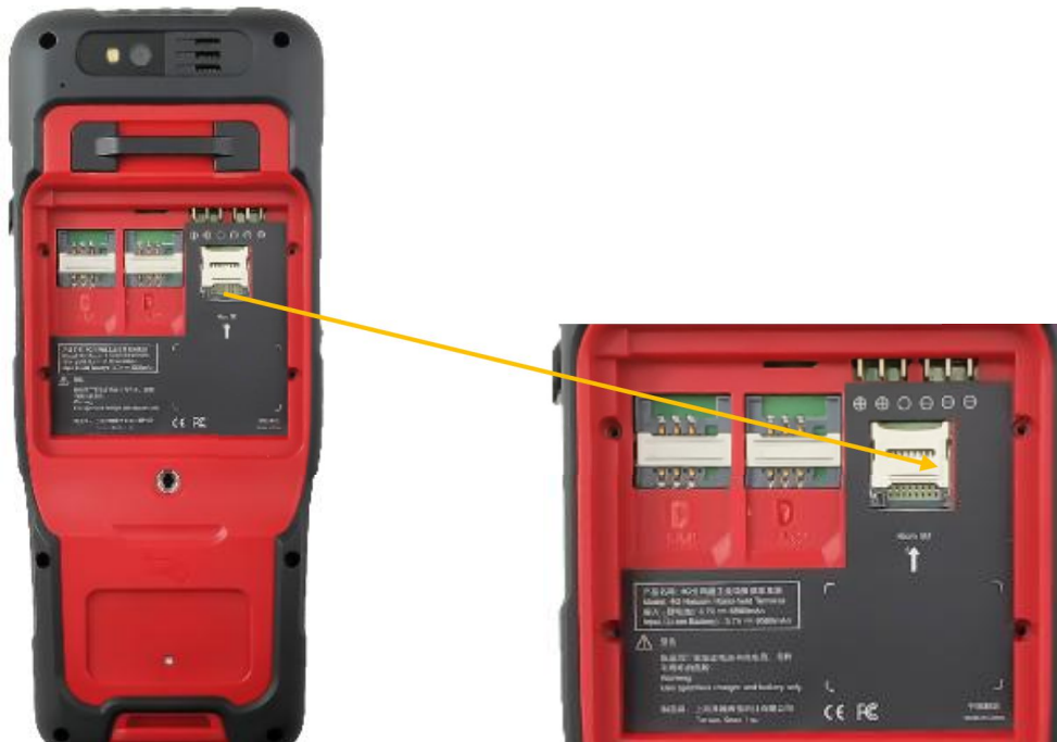
Figure 6.11 Insert Micro SD card
