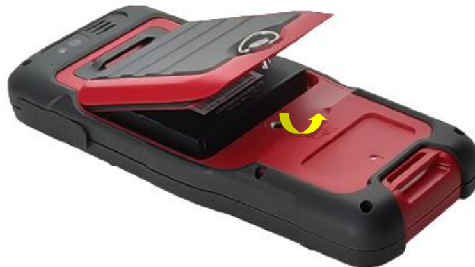
Figure 6.9 Take off the back cover
