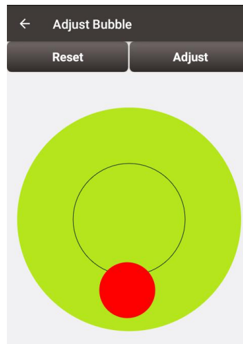
Figure 3.50 eBubble before adjusting
