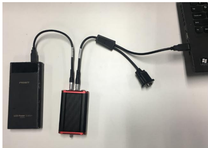
Figure 4.24 Connections of David, computer and power bank
