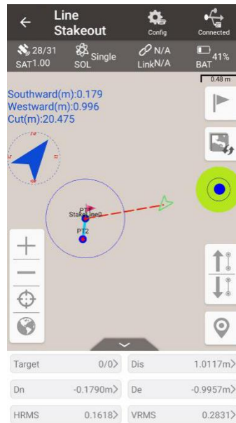
Figure 4.14 Line Stakeout interface
